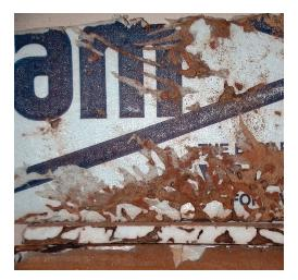
Figure 14. An example of foam-board insulation riddled with termite galleries. (B.T. Forschler)
