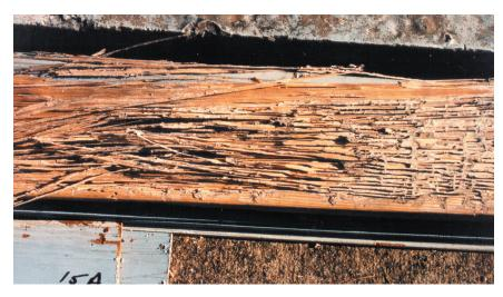
Figure 1. Subterranean termites excavate galleries in wood as they consume it, sometimes leaving nothing more than a thin wooden exterior. (B.T. Forschler)
